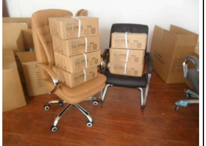
Loading test for 150kgs 2hours
